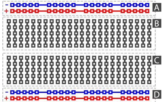
On both sides, there is two rails (for positive and negative) that run parallel. There are then 2 larger rails that run the power horizontally. Below you can see how the bread board cables run. [4]
