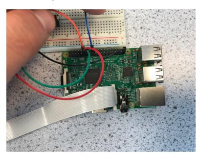
We want ground (black cable) to go to pin 39, switch to pin 12, green cable to pin 13, red to pin 11 and blue to pin 18. A diagram of the pin layouts is available in the appendix of this document.
