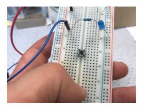
7. Plug in a black cable into port "g" horizontal to one of the legs. Plug the other end into the ground leg.
