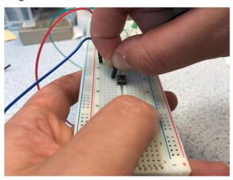
8. On column "G' plug the cable horizontally to the other leg of the switch. You should end up with the switch laid out such as:
