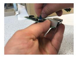
Push it in until the connectors are all in and secure. The raspberry pi will now start taking time lapse when turned on.
