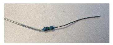
fixed resistor at 1K  $\Omega$  (omega). You can say which resistor which by their colours. For example 1K  $\Omega$  resistors have brown, 2 black followed by 2 red stripes on them as can be seen in the picture.
