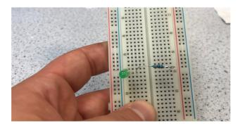
4. In the "J" column insert the corresponding colour cable for the LED.
